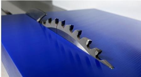
Thermoplastics are used in many different areas. Due to their different compositions, they are susceptible to melting, saw marks and edge breakages during processing.
