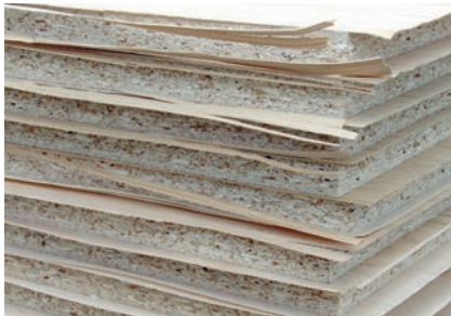
Example: Hogging of veneered panels with free veneer projection.
