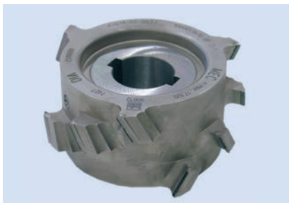
A) Conventional jointing cutter 91,5 dB(A).
