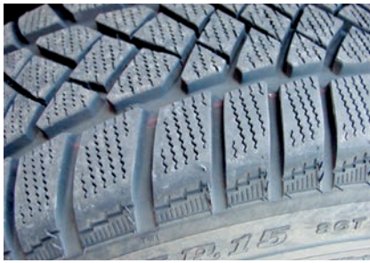
Tire profile with irregular pitch.
