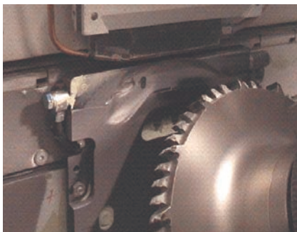
Problem: Machine wear through abrasive chips.
